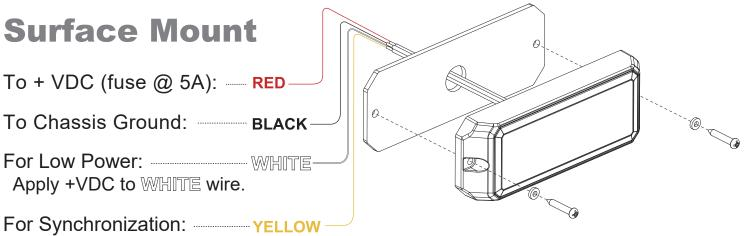
Connect YELLOW wires of all heads together for synchronization (All heads must be set at the same pattern)
